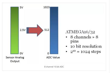
Suppose we use a 5V reference. In this case, any analog value in between 0 and 5V is converted into its equivalent ADC value as shown above. The 0-5V range is divided into  $2^{10} = 1024$  steps. Thus, a 0V input will give an ADC output of 0, 5V input will give an ADC output of 1023, whereas a 2.5V input will give an ADC output of around 512. This is the basic concept of ADC.
