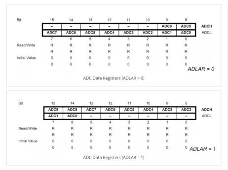
You can very well see the the effect of ADLAR bit (in ADMUX register). Upon setting ADLAR = 1, the conversion result is left adjusted.
