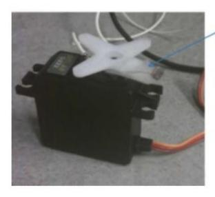
This is the light sensor, simply taped on, with wire wires going to the Butterfly
