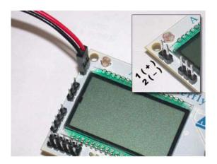
One side of the LDR would need to be connected to VCC and the other side would go to ground (the V- on the butterfly) through a pull down resistor (10K) with the analog signal coming from here to the AVR. See images below for connection examples from the data sheet(**Note** in the example below, the AVR Butterfly would take the place of the Arduino and you can use any VCC connection on the butterfly for the red wire)..
