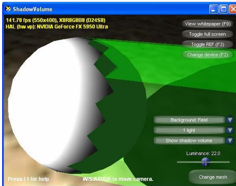
Figure 24: Displaying the shadow volume reveals that the jagged edge is caused by faces that are treated as being entirely in shadow when they are actually only partially shadowed.
