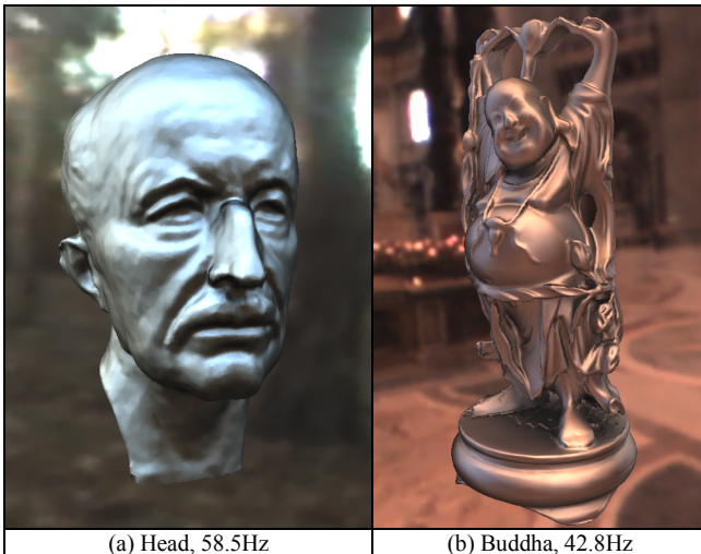
Figure 8: Glossy phong models. We get a performance speedup of 16-20x over the method in [Sloan et al. 2002] without noticeable degradation, by encoding with CPCA and using least-squares optimal projection to reduce matrix rows from 25 to 16.
