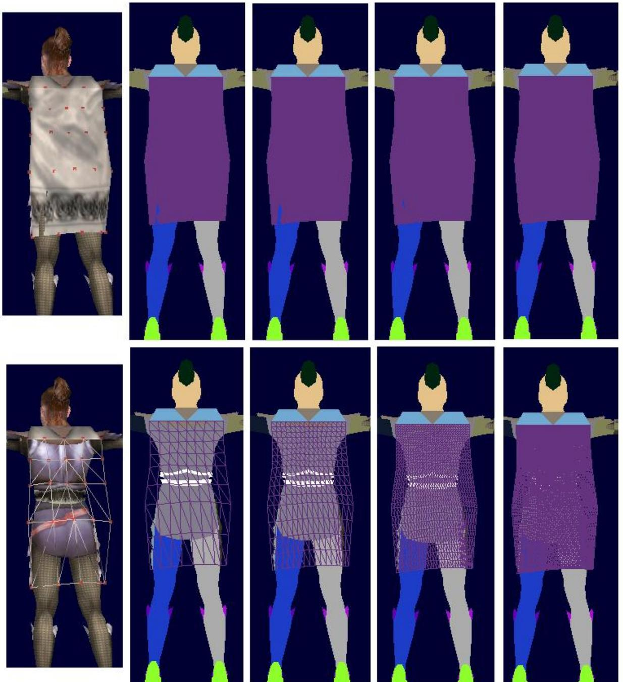
Figure 7.2: Collision is successfully detected and corrected in the finest mesh. Observe that collision is not detected until the second subdivision pass. This is because the cloth mesh is too sparse before the second pass and the newly added vertices are all on the correct side of the skin mesh.
