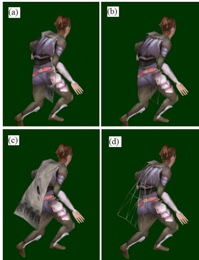
Figure 7.1: CPU Collision Detection and Correction Result. Image (a) and (b) shows the cloth motion before collision detection and image (c) and (d) shows the cloth motion after collision detection and correction. From the cloth mesh wireframes in (b) and (d), we can clearly see that the cloth vertices are corrected outside the body.
