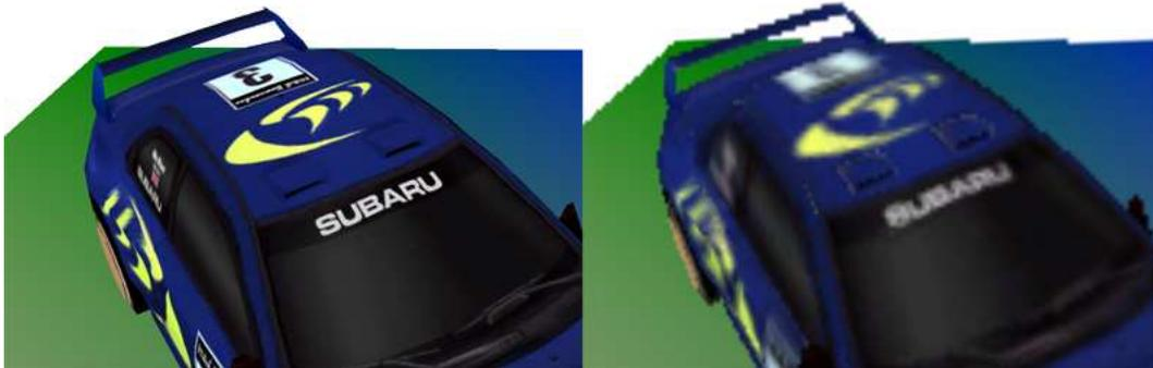
FIG. 4.11. Image quality comparison of the 12-microdisplay mapping example. The image on the left is directly rendered, whereas the image on the right has been created via mapping an original source image.
