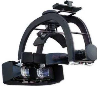
FIG. 4.1. Image of the piSight™ tiled HMD. Image used with permission from Sensics, Inc.
