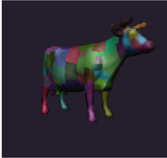
Figure 4.10: Global sampling rate. The grid distance is 0.01. The frame buffer resolution is 512 \times 512 .
