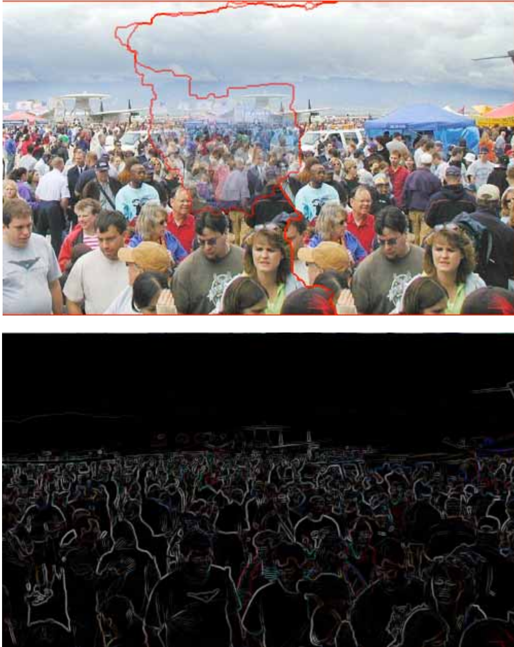
Figure 16: The top image shows the overlaying of the two different seams that were found by using edges and by not using edges. The bottom image shows the “edge map” that was used for determining where the edges were in the picture. Note that the edge map is only a single instance of the input image and that the results were truncated on the left hand side for size purposes.
