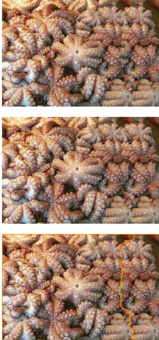
Figure 20: An example of using the old graph set up vs the new graph set up. The top image is cut using the old metric and the middle image using the new metric. The bottom image shows the seams for each image. The red represents the new metric and the yellow represents the old metric.
