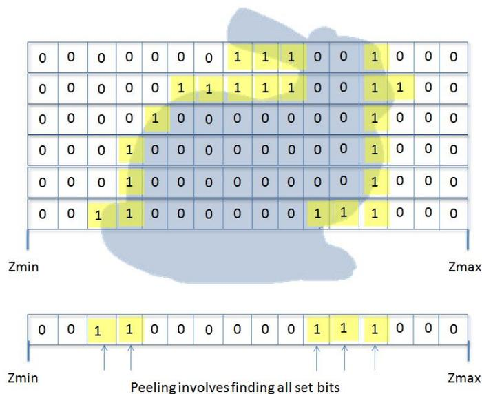
FIG. 3.1. Illustration of voxelization of the bunny model into 16 slices. Peeling depth layers simply involves finding the index of each set bit. A binary search can be performed to find each set bit
