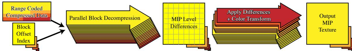
**Figure 2:** Overview of GPU decompression algorithm. Each bundle of arrows is a parallel GPU compute kernel
