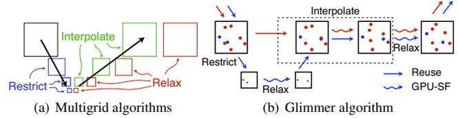
Fig. 1. **a)** The multigrid *v-cycle*. **b)** The Glimmer multilevel algorithm. The restriction operator builds the hierarchy by sampling points. GPU-SF is used as the relaxation operator at each level, with all points allowed to move, and as the interpolation operator, with only new points allowed to move. Lower levels untwist complex layouts while higher levels converge quickly because of computation at the lower levels.
