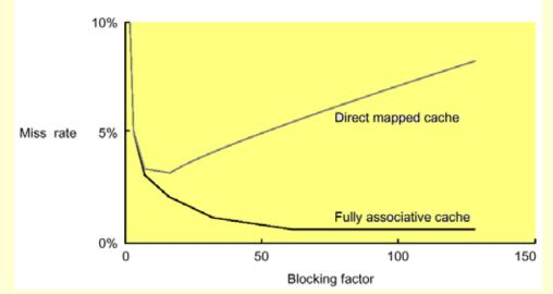
Lam et al [1991] a blocking factor of 24 had a fifth the misses compared to a factor of 48 despite both fit in cache
