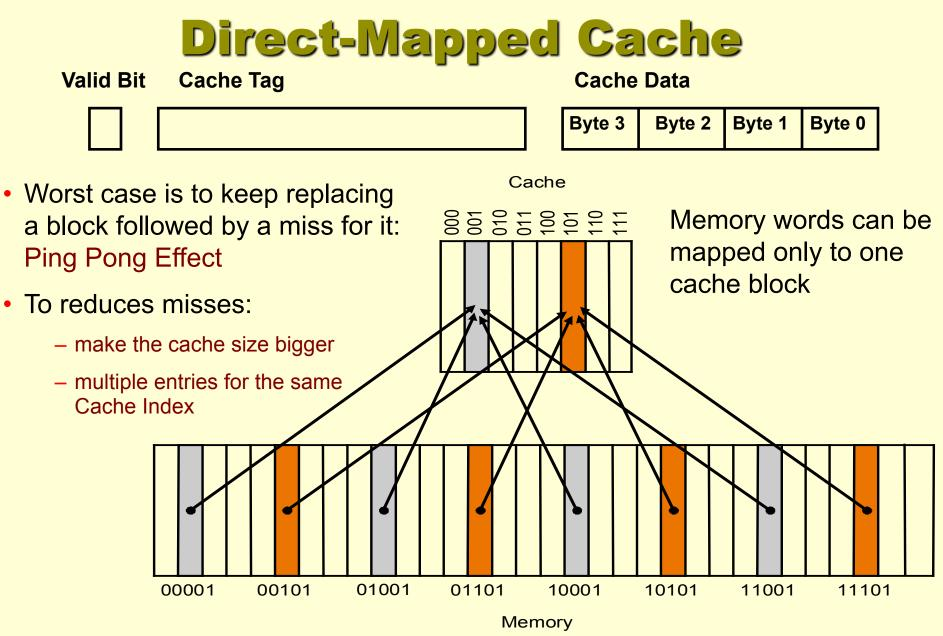
Cache block address = (Block address) modulo (Number of cache blocks)
