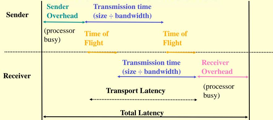
Total latency = Sender Overhead + Time of flight +  $\frac{\text{Message size}}{\text{Bandwidth}}$  + Receiver overhead
