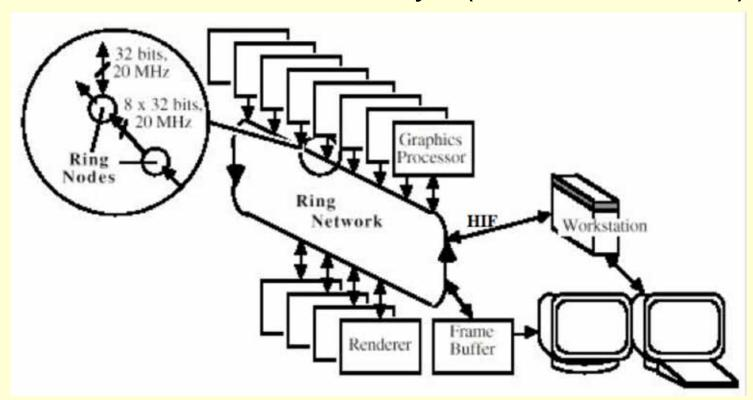
Fuchs, et al., "Pixel-Planes 5: A Heterogeneous Multiprocessor Graphics System Using Processor Enhanced Memories", SIGGRAPH 89
