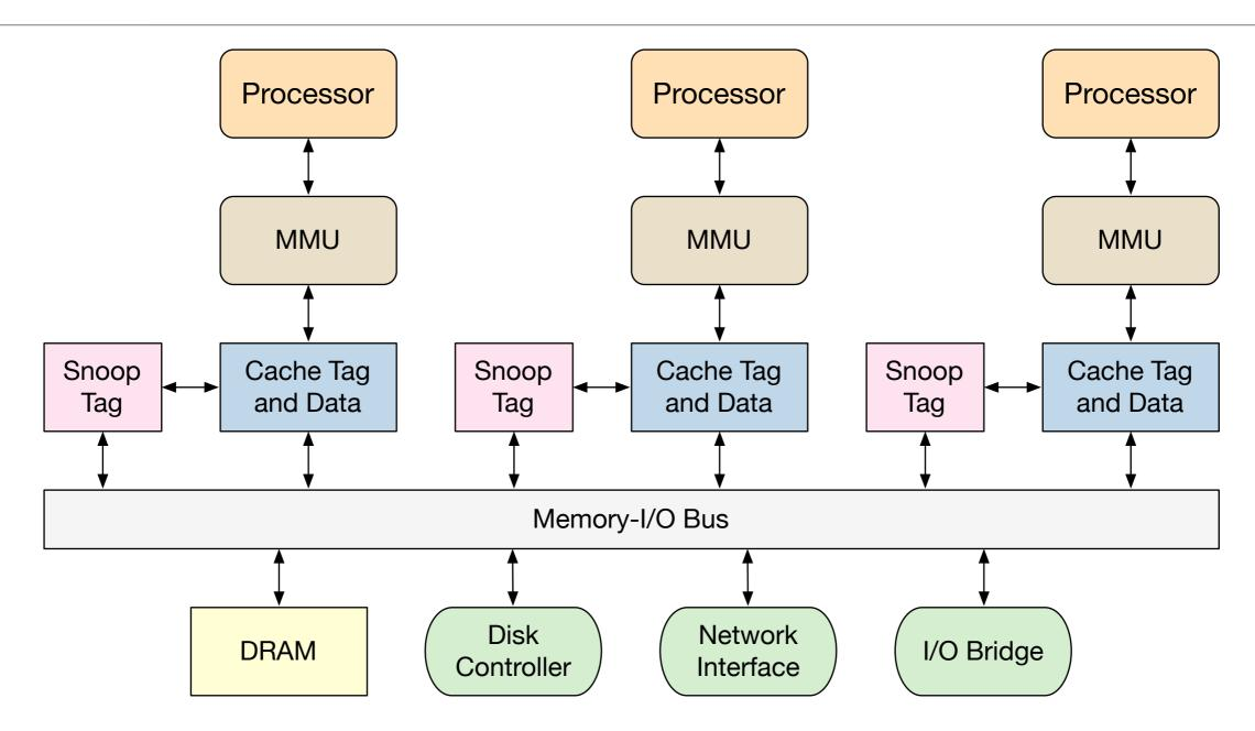
• Bus: shared communication link, using a set of wires to connect multiple subsystems
