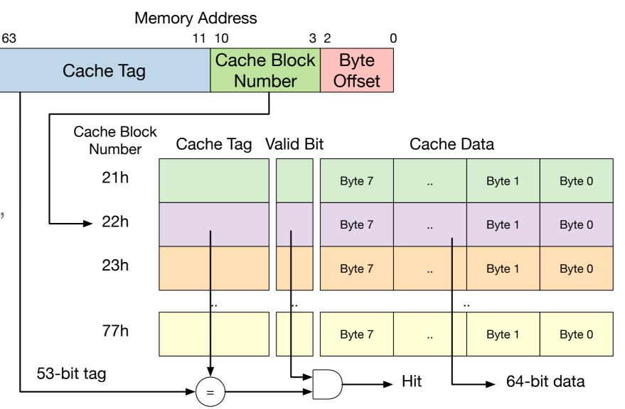
Total cache size is 30208 bits, of which 16384 bits (2048 bytes) are cached
