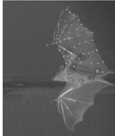
Figure 1: Frame from the video recorded by one of the three high-speed digital cameras. The 3D coordinates of markers attached to the bat wings are reconstructed using Direct Linear Transformation.
