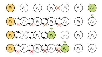
Fig. 1. Failure detection in ODSBR.
