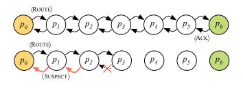
Fig. 3. BR1 message flow. The figure (for the failure case) shows only one possible failure scenario.
