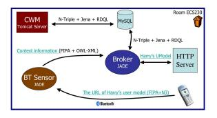
Figure 3: In our prototype system, the broker attempts to infer the location context of devices and users. An user model is dynamically acquired from an URL specified in the received user policy.
