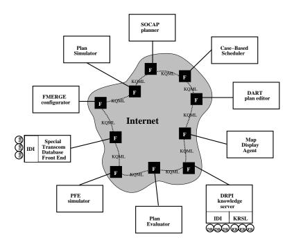
Figure 5: A network of processes communicating using the SKTP architecture is envisioned as a part of the DRPI testbed. Communication among the processes is handled by *communication facilitators*.
