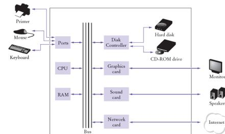
Figure 5 Schematic Diagram of a Computer
