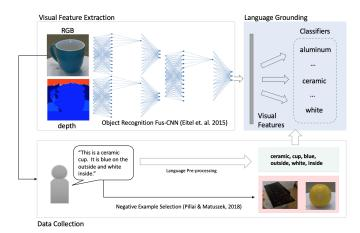
Fig. 2: Our proposed domain-free model using the visual features from object recognition system [7], creating word-asclassifier models. This method fuses two CNN architectures for RGB and depth images into fully connected fusion layers. We remove the softmax layer from their approach, exposing rich multimodal features for learning groundings.
