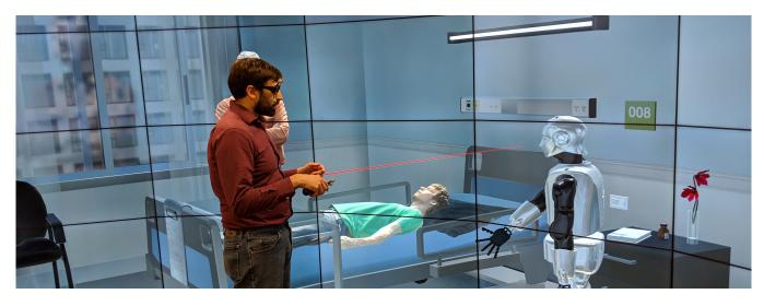
Figure 1: Using a monitor wall to talk to a virtual robot, modeled using a combination of Unity, ROS, and Gazebo.
