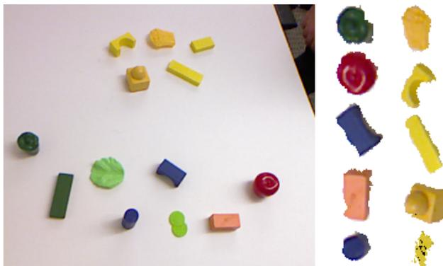
Figure 6.2: An example of an RGB-D object identification scene. Columns on the right show segments, identified as positive (right) and negative (center).
