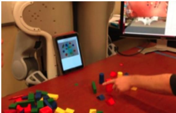
Figure 8.1: A data collection participant indicates objects to the PR2 robot “Rosie2.” The experimenter places an iPad with target objects circled in order to avoid linguistic or gestural priming. Part of the experimental user interface is shown (top right of image).
