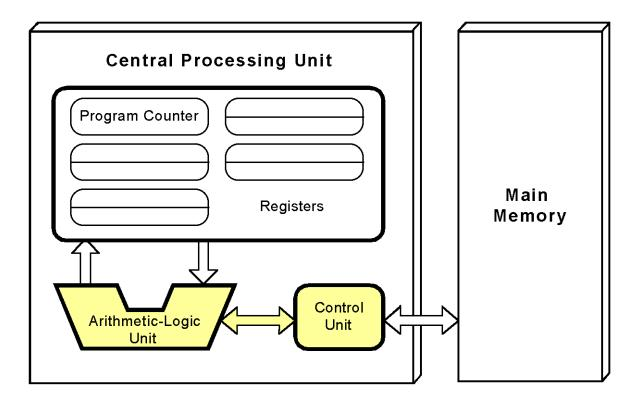
Any data operands required to execute the instruction are fetched from memory and placed into registers within the CPU.
