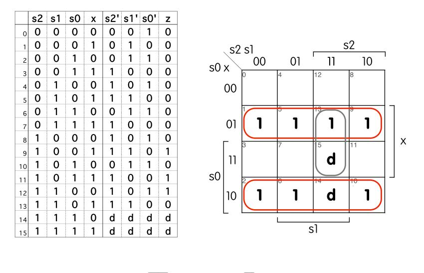
$s1' = \overline{s0} x + s0 \overline{x} = s0 x r x$
