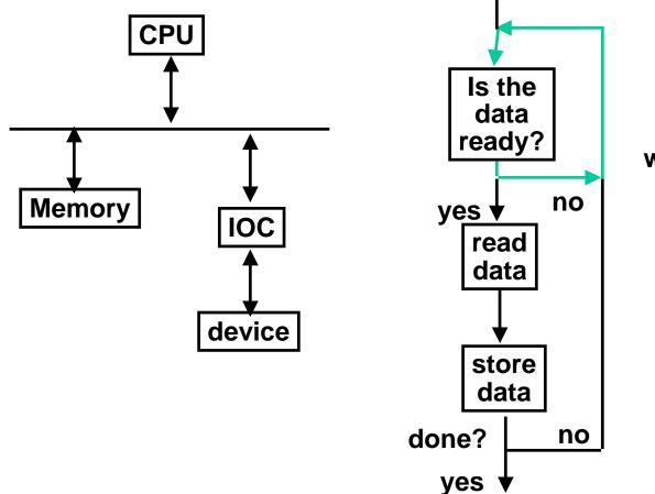
busy wait loop not an efficient way to use the CPU unless the device is very fast!
