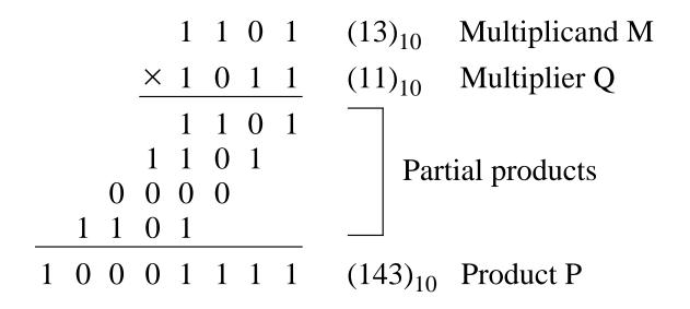
Multiplication of two 4-bit signed binary integers produces only a 7-bit result (each operand reduces to a sign bit and a 3-bit magnitude for each operand, producing a sign-bit and a 6-bit result).
